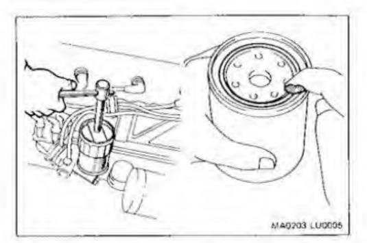
(b) Using SST, remove the oil filter (located on right side of engine block).
